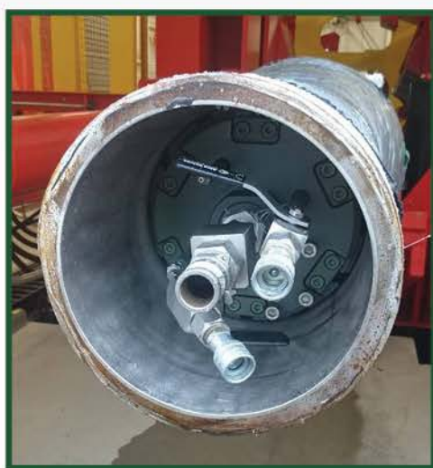
I-PEP™ installed in end of pipe stalk
