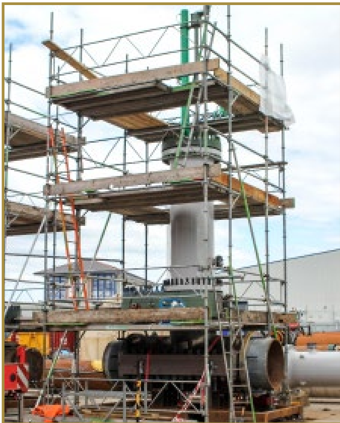
38" BISEP™, Slab Valve and Hot Tap Clamp during Factory Acceptance Test
