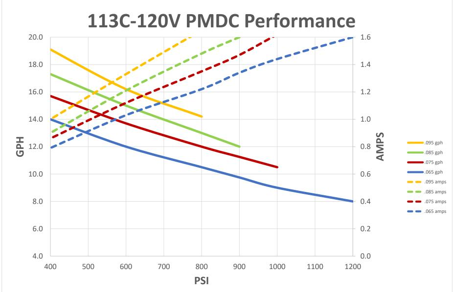
Data recorded pumping water at room temperature and rectified 115VAC power. Performance will vary with voltage fluxuations, application, and mfg tolerances. Copyright Pumptec Inc. 2020
