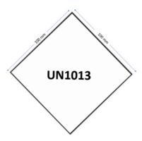
The "UN 1013" marking must be displayed within a square-on-points shaped area surrounded by a line that measures at least 100mm by 100mm on each side except for a single cylinder package. For these packages, the mark may be reduced to 30mm on each side.
