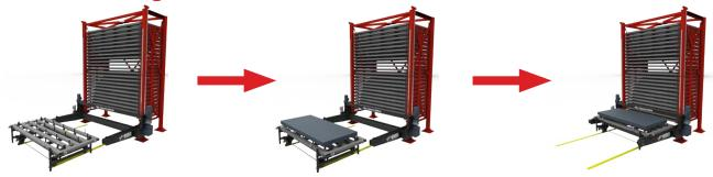
1. Place an empty pallet on the loading table/cart. If required, direct the pallet and cart in the necessary direction to the desired loading position.
