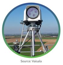
Light detection and ranging (LiDAR) systems can be mounted on top of the nacelle to gauge wind direction in front of the rotor. LiDAR uses laser beams directed upwind of the turbine to determine wind speed and yaw misalignment.
