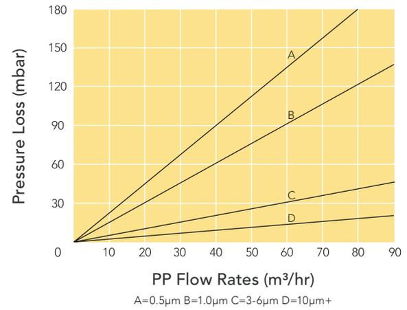
\*1 Amazon Filters recommend that SupaPleat HFC SRP cartridges are changed at a differential pressure of 1.5 bar in normal service - the operating conditions above should be treated as maximum differential pressures for short term use without causing cartridge collapse problems.
