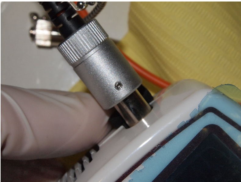
Figure 2: A NIR 915 nm diode laser has been used for the treatment. The SMA905 connection of the POCKET LASER device (88Dent PERO-MI) enable the quick substitution of cables and devices connected to the main unit.
