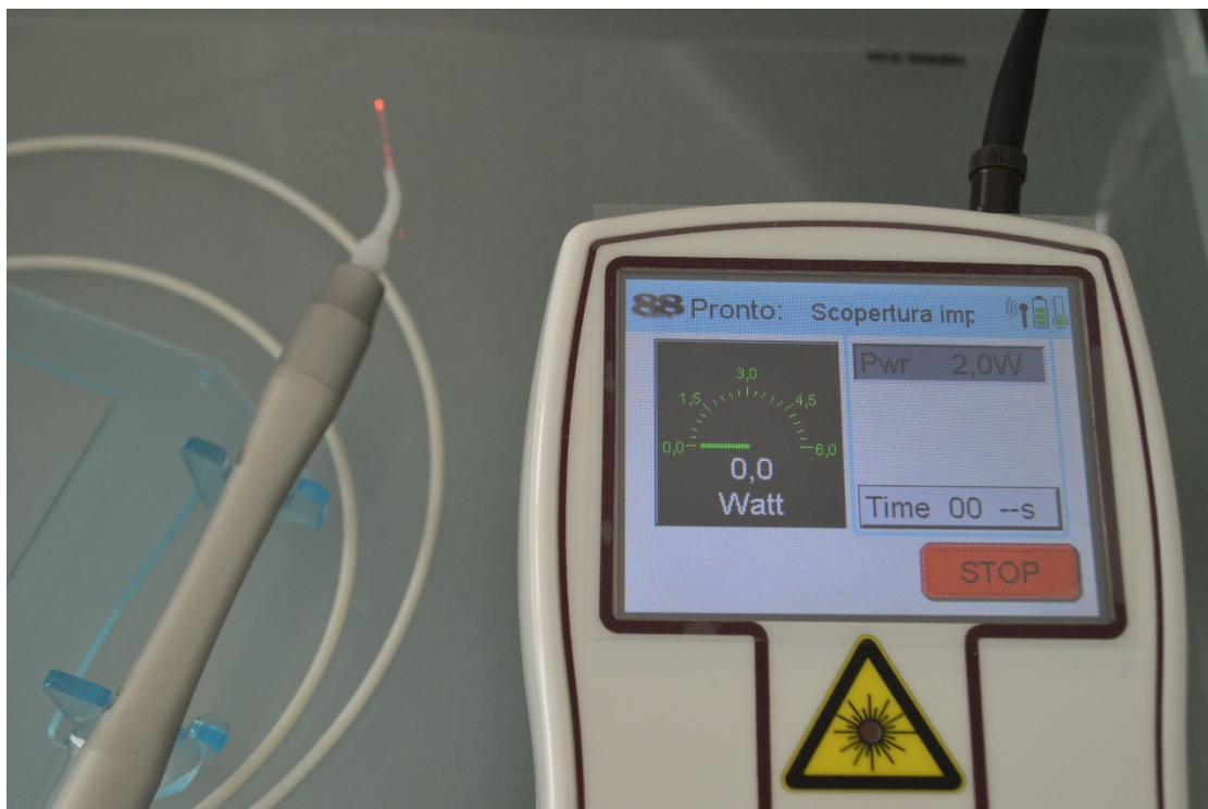
Figure 5 Either 200; 300 or 400 \mu m optical fibers can be used. During procedure a counter shows on display emission mode, power applied and time required.
