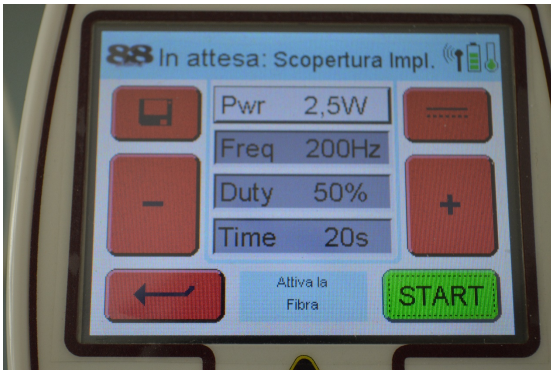
Figure 4 SOFT IMPLANT UNCOVERING PROGRAM ; PW 200 Hz 50 % Duty suitable in case of topical anaesthesia(or without anaesthesia) and thin periodontal-gingival biotype. Optical fiber initiation/activation is required.
