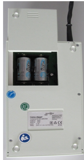
batteries in the battery compartment
