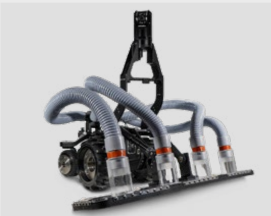
Raise and lower vacuum head 40 degrees
