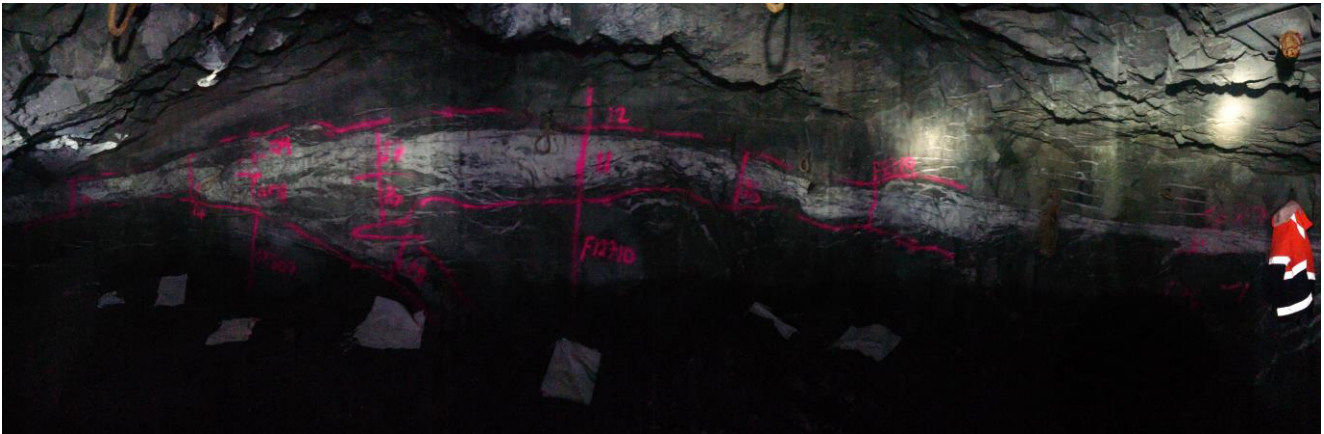
Fig (4): Face samples marked up 7 Level, Panel #1 North Ore Drive (NOD).
