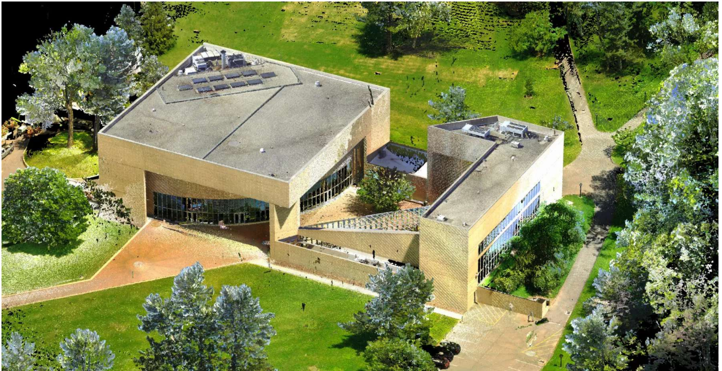
3D Laser Scan Data and 3D Revit Model, including exterior shell, floor plans, roof plans, reflected ceiling plans
