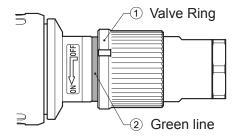
2 Attach the Connecting Hose to the tool, then turn the Valve Ring counterclockwise (4) while pushing the Valve Ring in the direction of 3
