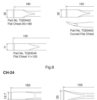
Part No. TP15234 Straight Flat Chisel 12.7×165mm
