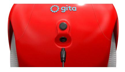
Make sure the center arrow on the charging cable aligns with the gita charging port before inserting.
