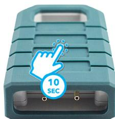
If the wayCOUNT device appears to be frozen or non-responsive, you can try to re-start the device. To re-start the device, press and hold the bottom button for 3 seconds.
