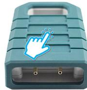
Press the button on the wayCOUNT device to put the device in pairing mode, your wayCOUNT device will be discoverable for the next 20 seconds
