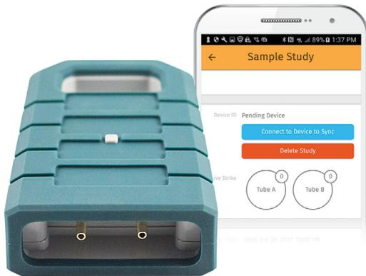
After pairing the study to the wayCOUNT device and connecting road tubes (see section 2 for proper road tube installation, you can see the Live Strike of each road tube. If you do not see the Live Strikes occurring when cars are driving over the tube (or during simulation) reconnect the device and it should appear.
