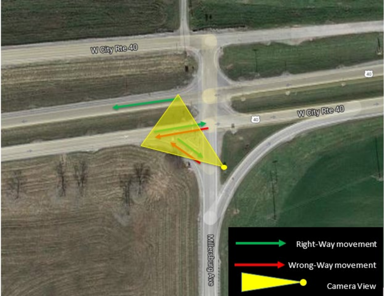
Figure 3.1 Camera Setup at Exit 41 Northbound on I-70.
