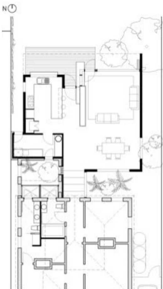
Floor Plan Existing House & New extension
