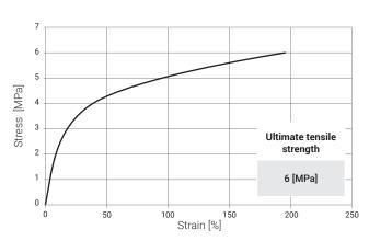
While the tensile stress does not exceed 3.0 [MPa], after load release, the test specimens retain their shape, with no external damage observed (e.g. fractures). The test specimens fracture when a max tensile stress of 6 [MPa] is applied.
