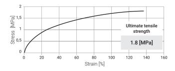
While the tensile stress does not exceed 0.8 [MPa], after load release, the test specimens retain their shape, with no external damage observed (e.g. fractures). The test specimens fracture when a max tensile stress of 1.8 [MPa] is applied.
