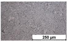
Microstructure after hot isostatic pressing (HIP)
