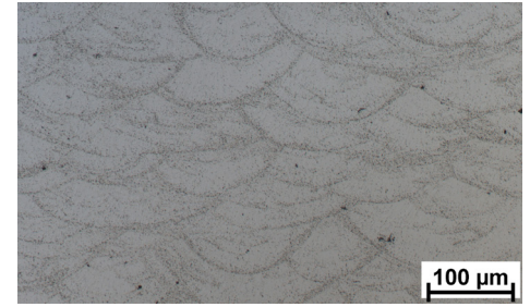
Microstructure after SR
