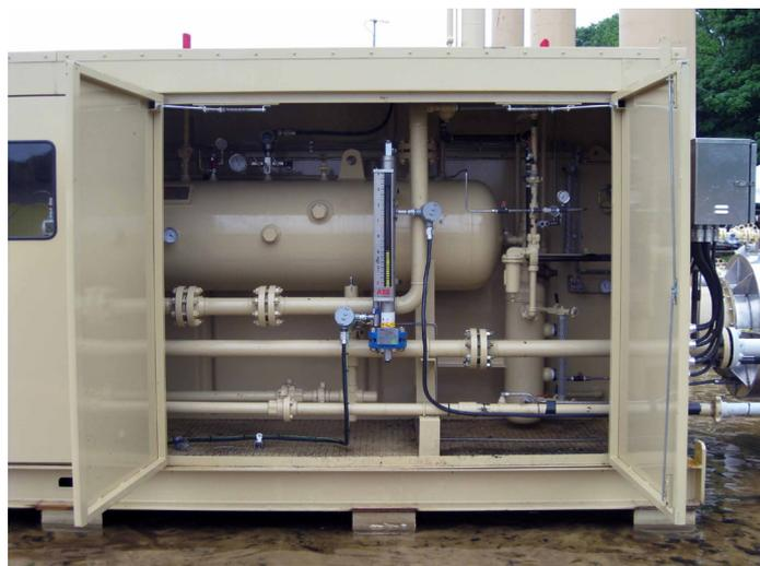
switch to sense the fluid height, which would signal a solenoid to open and close a dump valve. Fluid overflow would often occur due to the inaccuracy of the pneumatic devices as well as the slower response time of the antiquated technology. A level solution was needed to separate water from the GPU, and maintain the customer's specific set points so that precise flow measurement could be achieved without water reaching the sales line.
