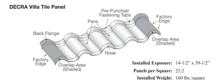
Villa panels are not designed to be installed over irregular surfaces.
