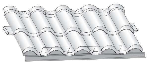
Install Villa Bird Stop - Eave and fasten through the front edge of the panel, off to one side of the low point
