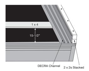
**Panels - First Course:** Fasten the first course of panels through the pre-punched fastening tabs to the 1 x 4s using minimum #9 Hex (1/4" hex head) x 1-1/2" long screws that will fit flush to panel and are long enough to penetrate the deck securely.
