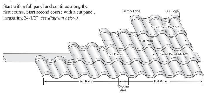
Measure panels and make cuts accordingly so the cut edge starts (or terminates) in the DECRA Channel or Villa Valley (see diagram below). Panels can be cut from either side (see diagram right). Save cut-off pieces for use on opposite side terminating into Villa Valley or DECRA Channel.
