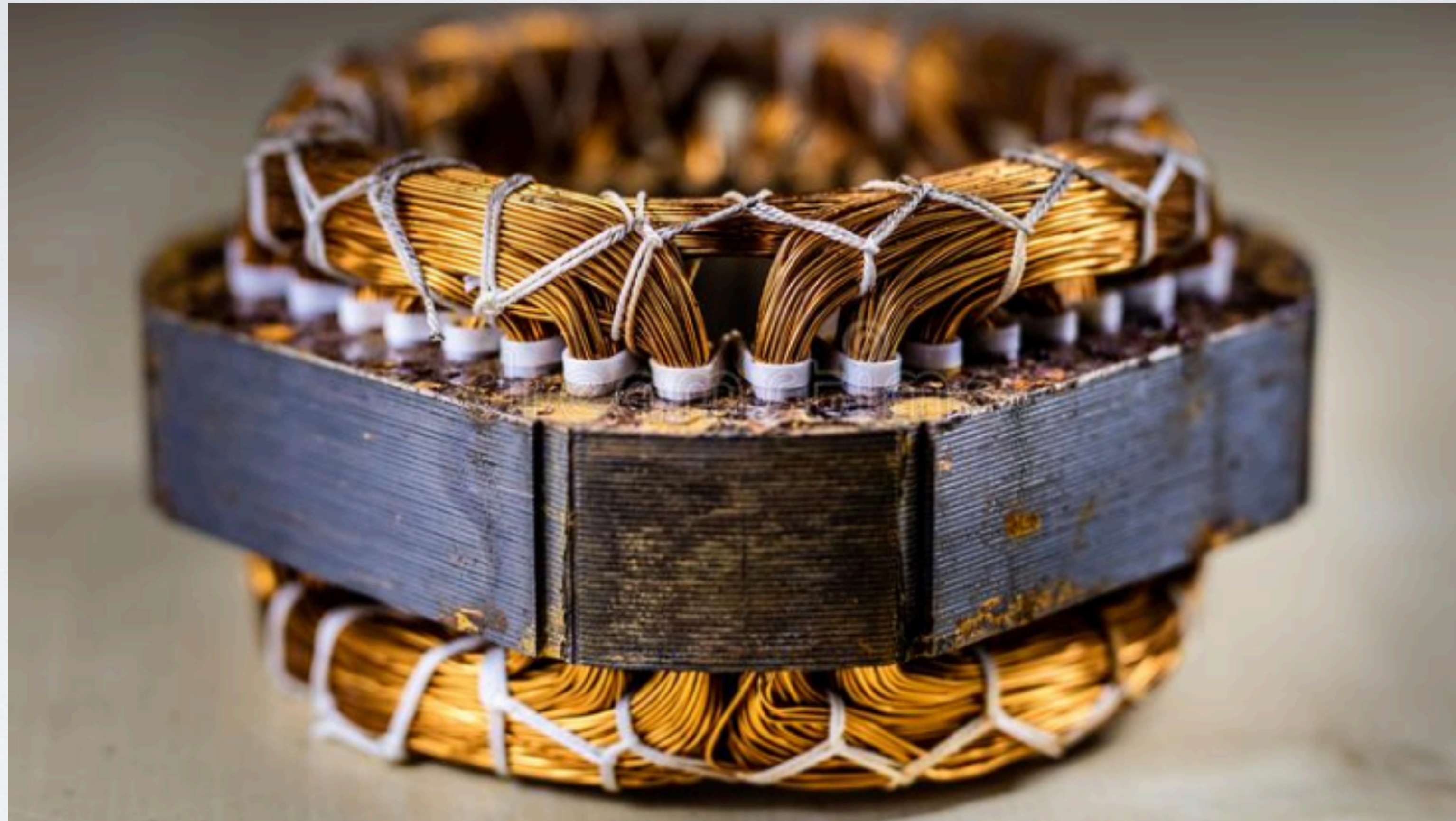
Century old copper wound iron core stator
