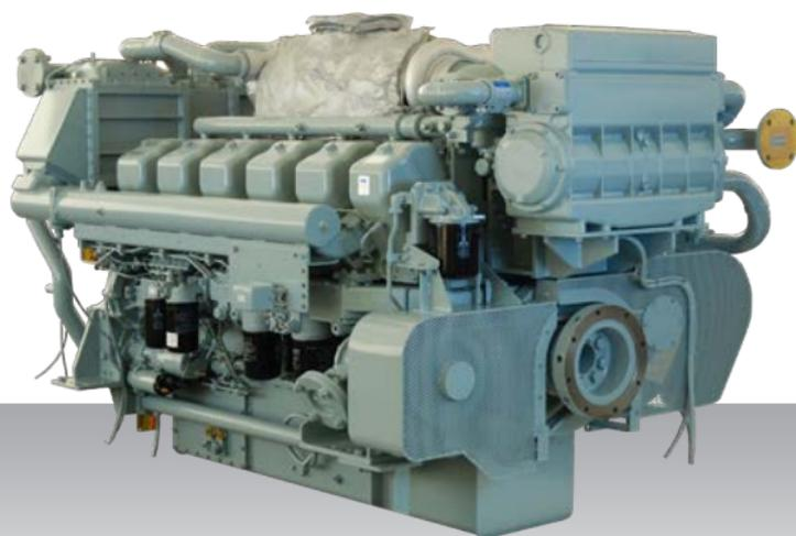
12-cylinder, 4-stroke, water-cooled diesel engine, with direct-injection, turbocharger, air-cooler, built-up heat exchanger and sea water pump.
