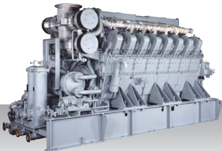
16-cylinder, 4-stroke, water-cooled diesel engine,
