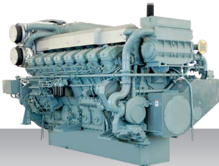
16-cylinder, 4-stroke, water-cooled diesel engine, with direct-injection, turbocharger, air-cooler, built-up heat exchanger and sea water pump.
