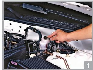
2. Place the refill pot, which contains new brake fluid, into the reservoir. New fluid will automatically flow in to keep the level constant.
