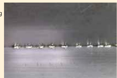
Corner spot welding thickness 0,6 mm
