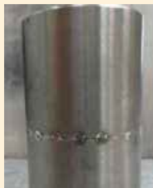
Pipe butt weld Ø 31.75 x 2 mm
