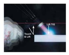
The Invertec® V205-S features "Lift TIG" as standard and enables the welder to start the TIG arc by lifting the tungsten electrode from the work piece without tungsten contamination or the need for H.F. ignition.
