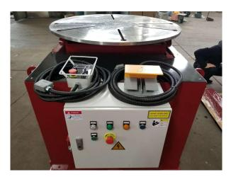
E-Stop switch install side of the machine, to ensure the safety.
