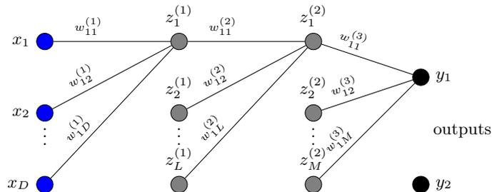
Fig. 2: MLP architecture. For clarity the diagram displays connections for a few units. Each layer is fully connected with ReLU activations. Input dimensions  $D = h_1 \times w_1$ . Number of hidden units in the first and second layers labelled  $L$  and  $M$  respectively.
