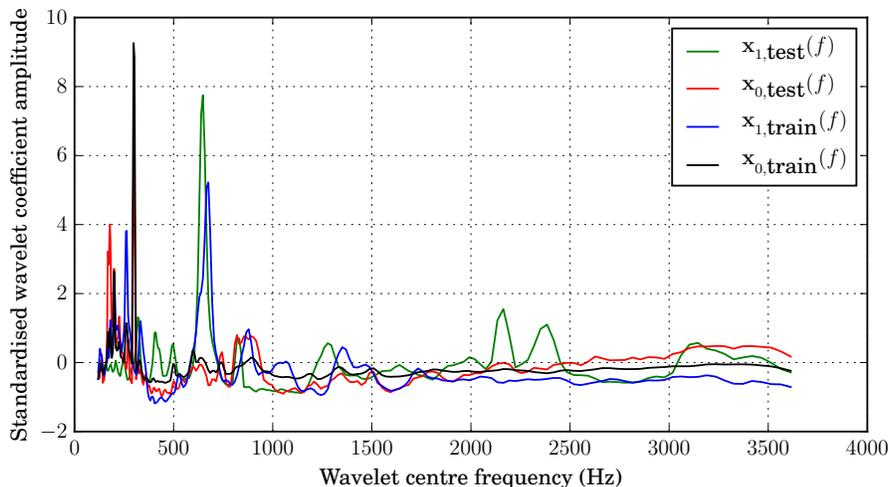
Fig 5: Plot of standardised wavelet coefficient amplitude against centre frequency of each wavelet scale for the top 10% predicted outputs over a test dataset. The learned spectra  $\mathbf{x}_{i,\text{test}}(f)$  for the highest  $N$  scores closely match the frequency characteristics of the labelled class samples  $\mathbf{x}_{i,\text{train}}(f)$ .
