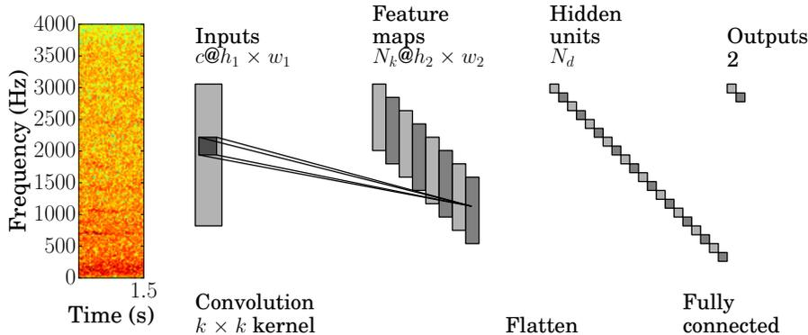
Fig. 1: The CNN pipeline. 1.5 s wavelet spectrogram of mosquito recording is partitioned into images with  $c = 1$  channels, of dimensions  $h_1 \times w_1$ . This serves as input to a convolutional network with  $N_k$  filters with kernel  $\mathbf{W}_p \in \mathbb{R}^{k \times k}$ . Feature maps are formed with dimensions reduced to  $h_2 \times w_2$  following convolution. These maps are fully connected to  $N_d$  units in the dense layer, fully connected to 2 units in the output layer.
