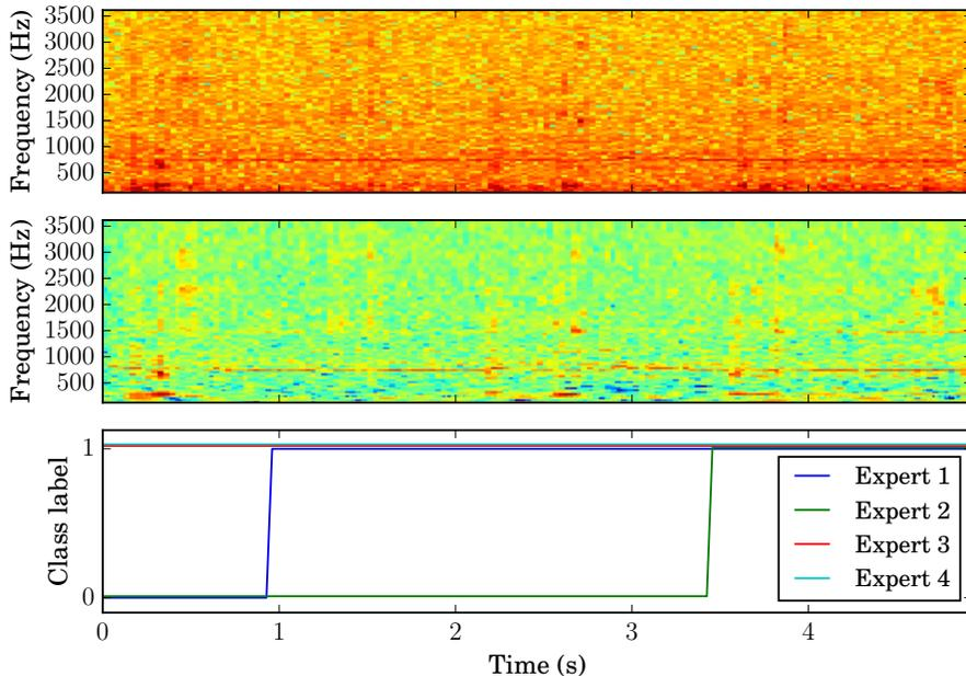
Fig. 3: STFT (top) and wavelet (middle) representations of signal with  $h_1 = 256$  frequency bins and wavelet scales respectively. Corresponding varying class labels (bottom) as supplied by human experts. The wavelet representation shows greater contrast in horizontal constant frequency bands that correspond to the mosquito tone.
