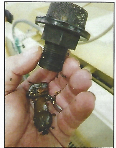
Figure 5 Replacing plugged Adsorption Clarifier nozzles enhanced performance
