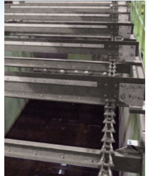
Pivoting chain-and-flight mechanisms were replaced with a fixed design.
