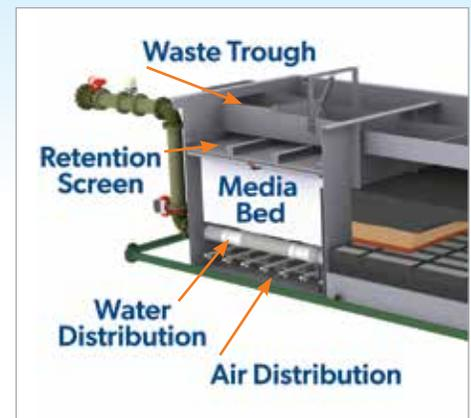
Cutaway rendering of Adsorption Clarifier unit
