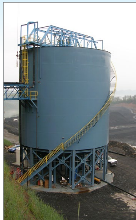
WesTech 15m diameter Deep Bed™ paste thickener located above the deposition site.
