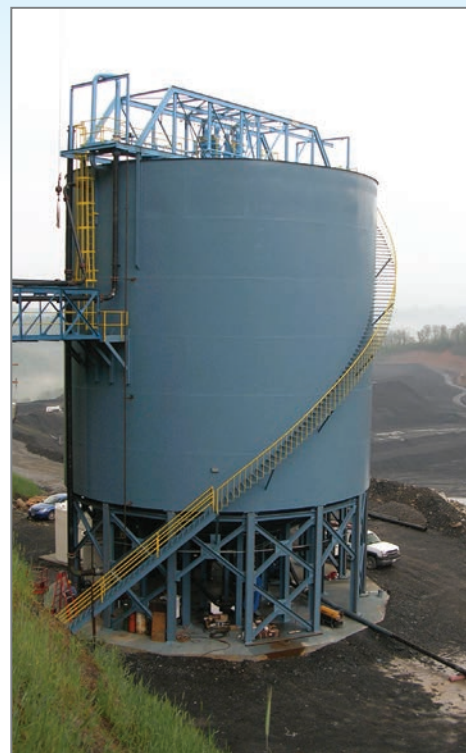
WesTech 15m diameter Deep Bed™ paste thickener located above the disposal site.
