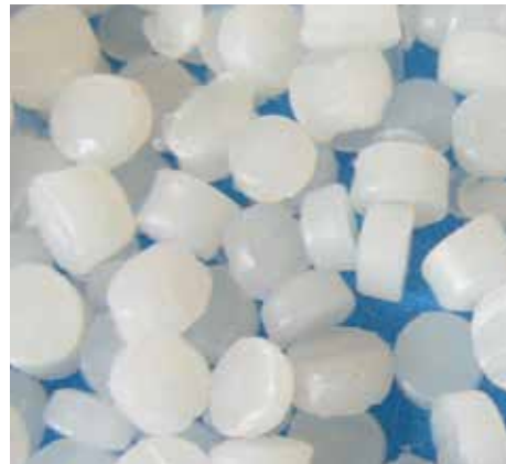
In the first stage, water flows upward through buoyant media, which provides flocculation.
