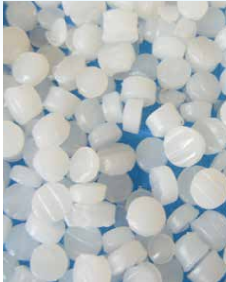
Adsorption Clarifiers use buoyant media in an upflow system design.
