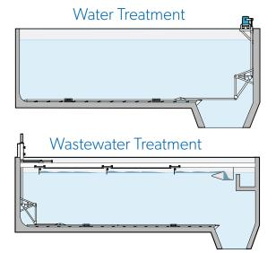
The ZICKERT Shark has been applied to numerous water treatment processes. The design of the mechanism provides a cost-effective stainless steel system. The mechanism can be set on a timer to allow for additional thickening of the chemical solids. The low profile of the mechanism makes it ideal when using plate or tube settlers.
