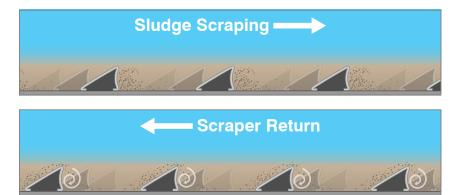
The wedge-shape on the back of the blade and the increased speed of the return stroke allow for minimal disturbance of the sludge blanket.
