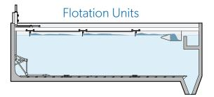
The effectiveness of the ZICKERT Scum Skimmer has proven to be a simple and reliable solution for dissolved gas flotation units and oil/water separators. The adjustable skimmer and float box provide the flexibility for solids removal. The ZICKERT Shark can be applied to pretreatment, thickening, or refinery processes.
