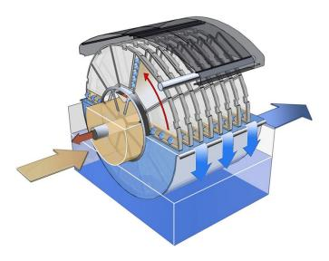
When the water level inside the filter rotor increases to a pre-set point, the filter rotor starts rotating and the backwash of the filter media starts. The high pressure backwash spray removes the accumulated suspended solids into the reject flume inside the filter. The suspended solids are then discharged via the reject pipe. The discs are submerged to approximately 65% and the water level of the filtrate is maintained by an integral outlet weir.
