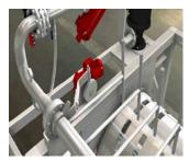
The oscillating spray bar backwash system and the integrated level tank are some of the specific design details that make the SuperDisc™ a reliable and low-maintenance filtration unit with more operational control.
