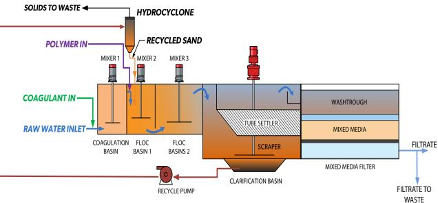
By combining two successful solutions, the RapiSand Plus provides a compact system with the capacity and performance of a larger system.
