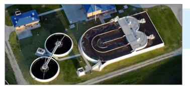
The OxyStream™ oxidation ditch system combines slow-speed surface aerators with an oxidation ditch design based on site-specific conditions and WesTech's proprietary hydraulic model.
