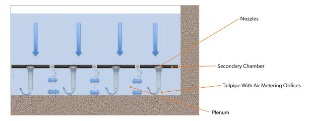
Backwash processes use the same nozzle and tailpipe system. Backwash water enters the filter cell through a flume. Orifices on the tailpipes meter air and water, which pass up to the secondary chamber, up through the surface slots
