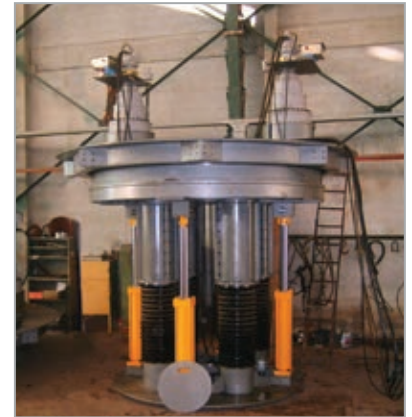
Cage Drive with Hydraulic Lift
