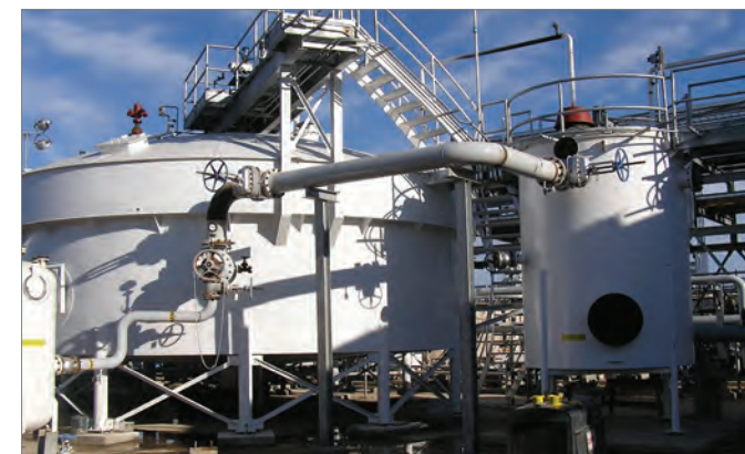
Circular DGF designs are used for higher flow rates while rectangular tanks offer higher residence time.
