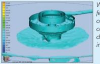
WesTech's EvenFlo<sup>™</sup> feedwell provides optimal flocculation conditions and even distribution of solids in the thickener.
