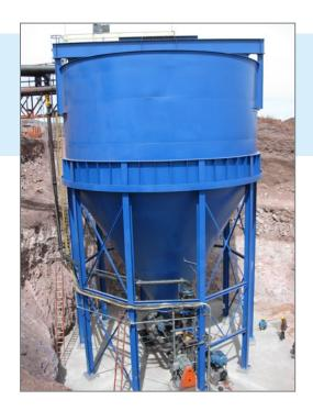
The AltaFlo<sup>™</sup> ultra high-rate thickener is a rake-less thickener that provides mixing, flocculation and internal dilution, followed by clarification and positive sludge collection and removal, all in a single tank. The principles of dewatering have been further optimized to a new design that thickens slurries at an even higher rate than a typical high-rate thickener.
