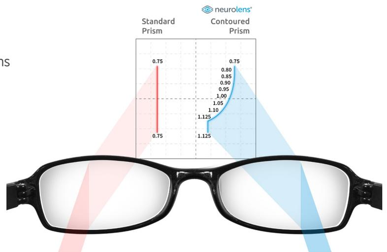
Contoured prism design provides more prism where it is needed most
