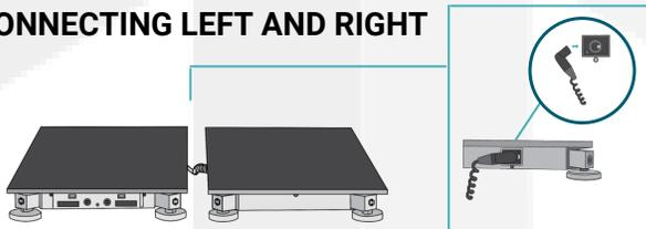
Connect your plates by aligning the cable with the receptacle on each plate, and press in until you hear a "**click**". To disconnect the cable, press the silver "**push**" button on the receptacle and gently remove the cable
