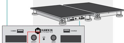
Turn the plates on by pressing the **ON/OFF** button on the control panel. The LED will blink in the boot sequence.
