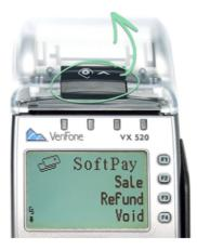
2. Drop the paper into the tray with the leading edge feeding down from the bottom of the roll.
